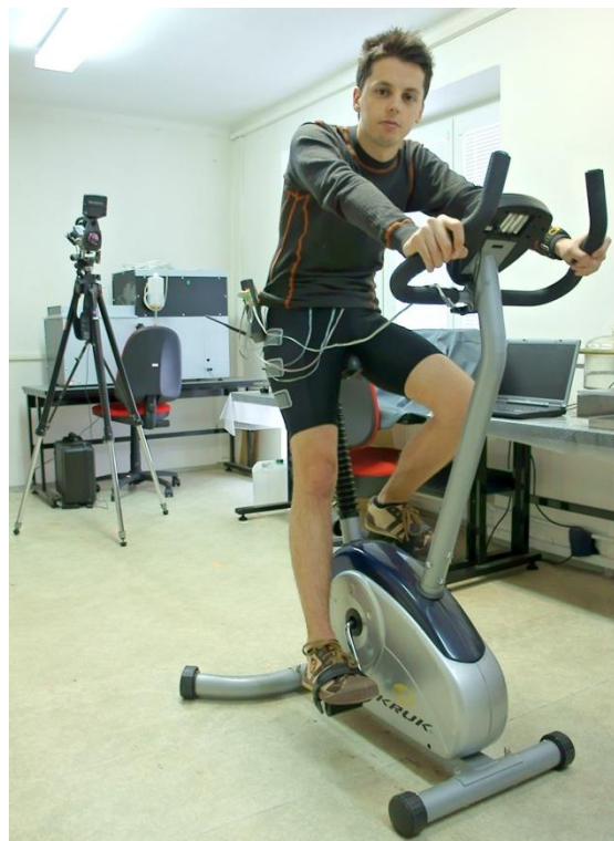
Fig. 1: Proband while testing the 1st layers of clothing in the laboratory of physiologic comfort.
