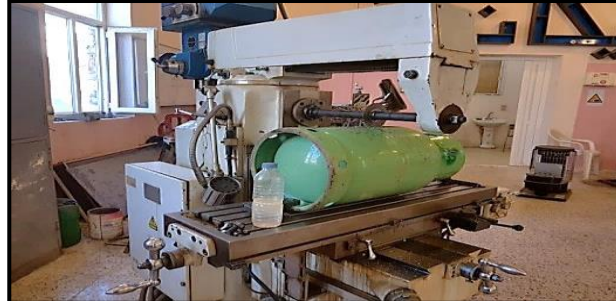
Fig. 6: Cutting process of LPG cylinders
