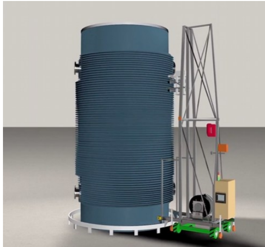
Fig. 1: Castor 440/84 and existing mobile radiation measurement system
