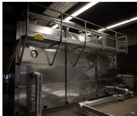
Fig. 1: Photo of the ZFT representing the containment sump of a PWR
