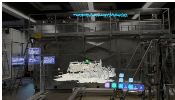
Fig. 14: See-through view of the AR application with the HoloLens 2 from two different perspectives including the flow simulation in blue
