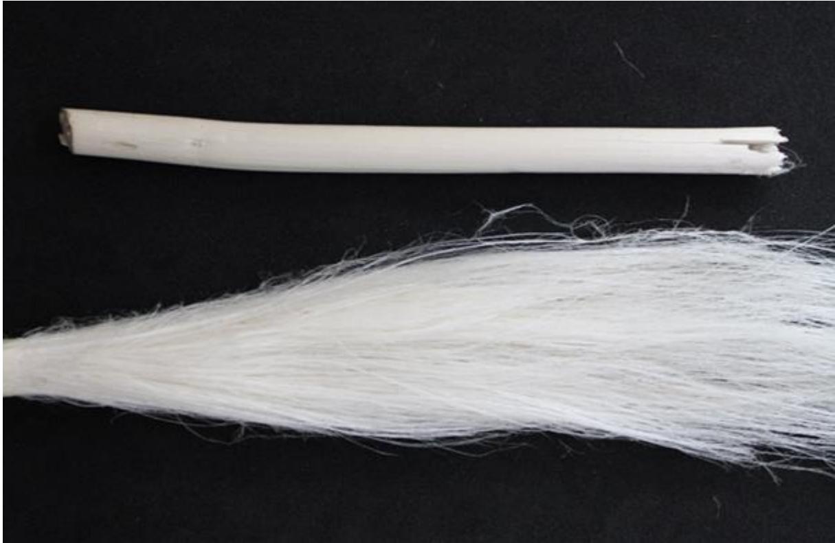
Fig. 6: Examples of hemp products after anaerobic digestion. As a result of water retting clearly separated fiber bundles without surface contamination and clean stalks (hurds) are obtained for further processing.
