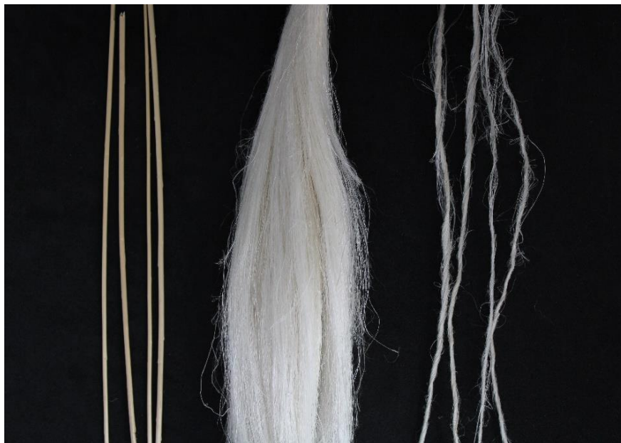
Fig. 9: Flax after anaerobic digestion. Flax stalk (left), flax fibers (in the middle), and flax yarn (right).
