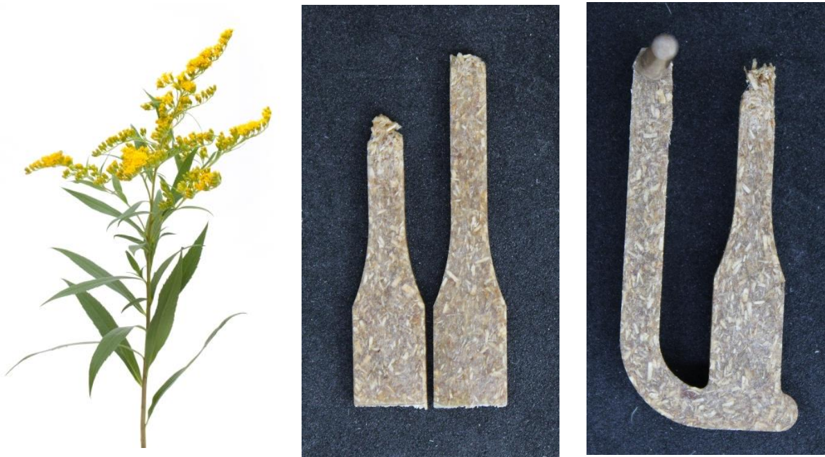
Fig. 10: Picture of goldenrod (left), tensile test bars with goldenrod (right)
