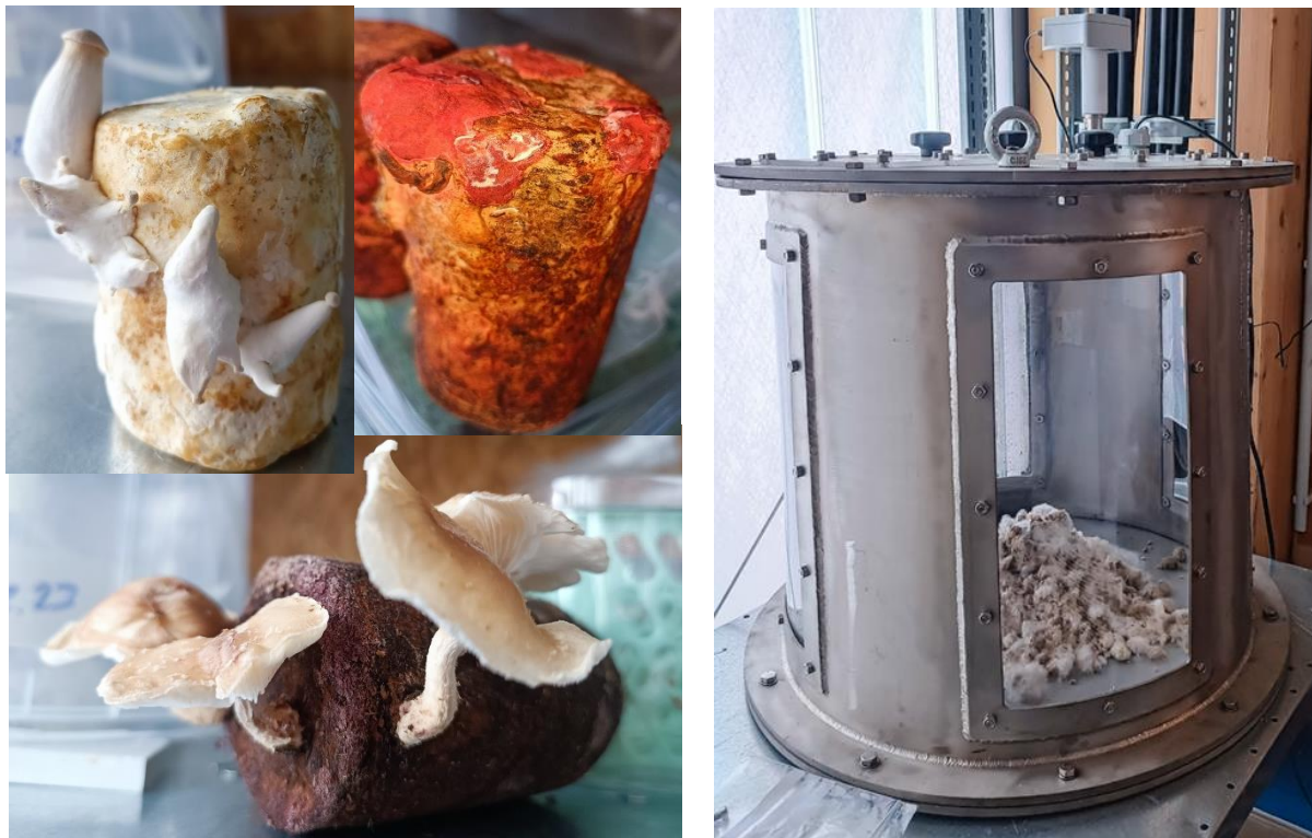
Fig. 12: Fungi growing on shreds of NFC parts. Pleurotus eryngii , Pycnoporus cинеbareus and Letinus edodes (left picture), Irpex lacteus in mycoreactor developed and produced in this project (right picture)
