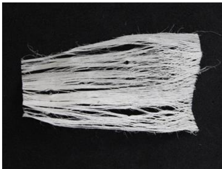
Fig. 11: Exposed mesh structure of fibers
