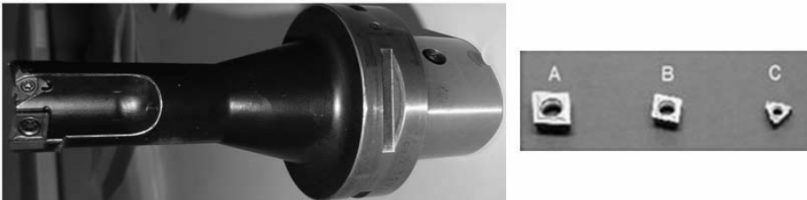
Fig. 5: FlashTool the Multi-Profession Tool with Three Types of Tool tips
