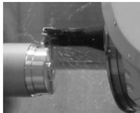
Fig. 7: 3D Model of the Sample Part and the Demonstration of the Machining by the Multi-Profession Tool - FlashTool
