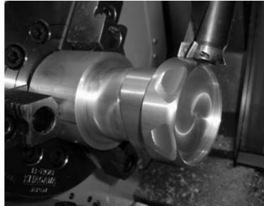
Fig. 6: Model 3D of the Sample Part and the Demonstration of the Machining by the CoroPlex MT Multi-Profession Tool
