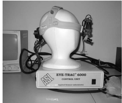
Picture 2: This picture shows the eye tracker
