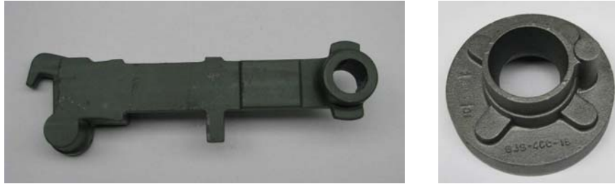
Fig. 1: Patterns of castings from ductile iron (lever and hub)
