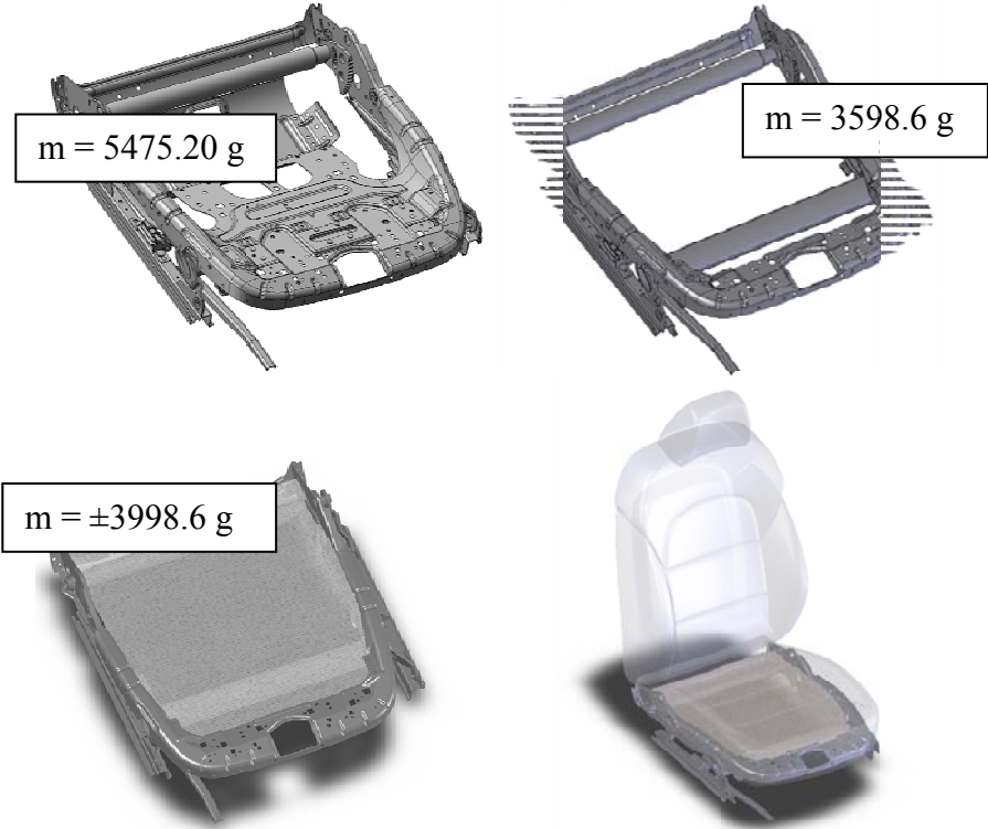
Fig. 1 Design with steel reinforcement, without steel braces, Substitute for viscoelastic composite material, Viscoelastic composite material applications in car seat design
