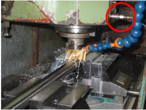
Fig. 1: Placement of the vibration sensor
