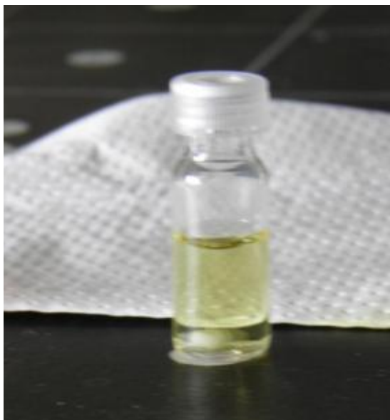
Fig. 2: Extraction of analytes from HCOOH into n-pentane after irradiation and deposition of the SC particles. The yellow color of the more dense formic acid phase is neither due to remaining nitroaromatics (reduction is complete) nor to metal ion dissolution but points to unidentified red to brownish organic decomposition products.
