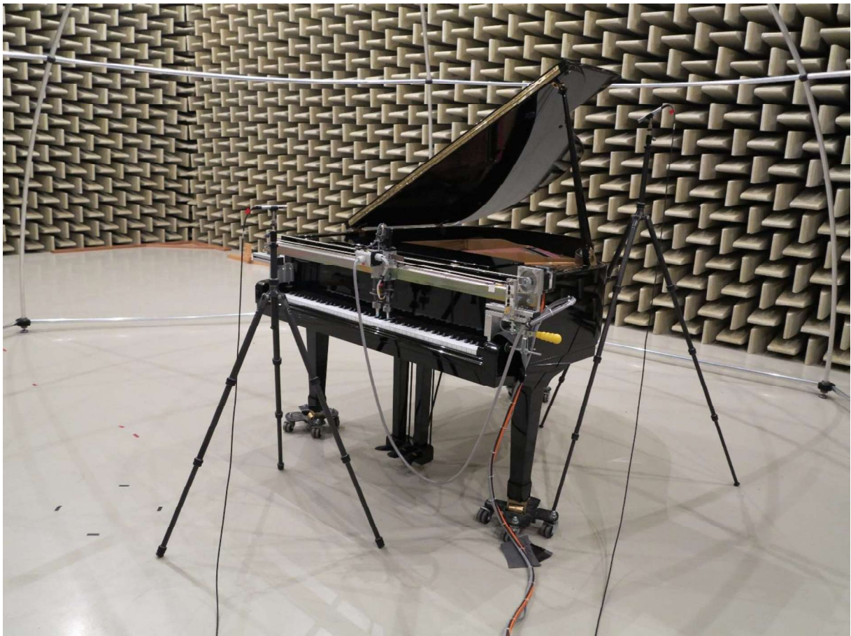
Fig. 3: The rebuilt and modernized play-bench
