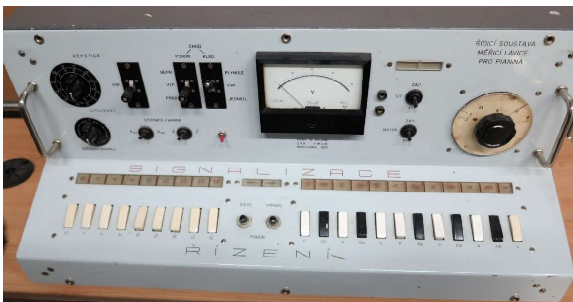
Fig. 2: The control system for measurement settings of the original play-bench
