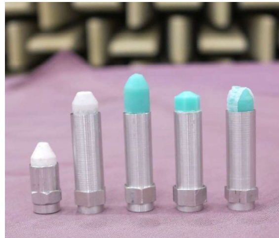
Fig. 6: The development of artificial fingers to the far left: original artificial finger made of teflon, to the far right: the final form of artificial finger made of addition silicone and teflon tapes
