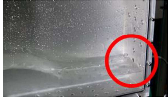
Fig. 5 (b): Moment of exposure of the pressure sensor about X - Z oscillation.
