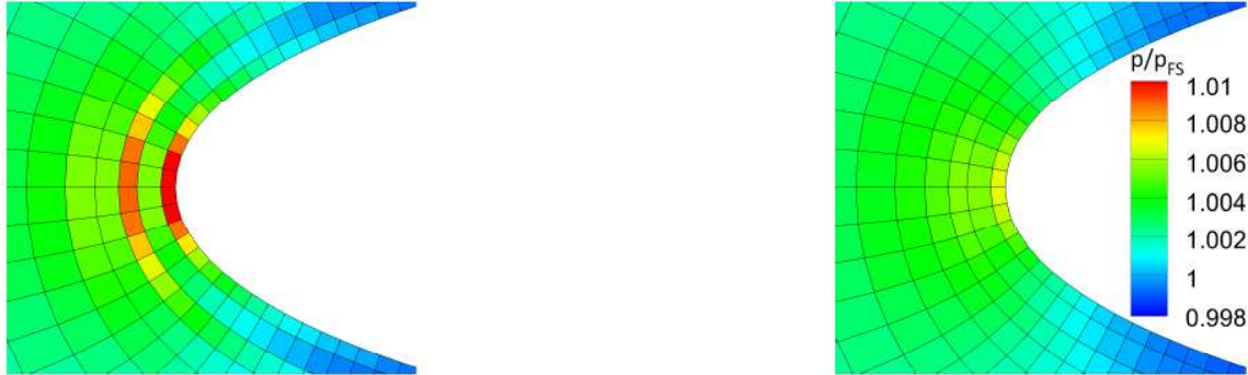
Fig. 4: Distribution of non-dimensional pressure near airfoil LE from AUSM + (left) and AUSM + -up scheme (right) for u_{1,FS} = 30 m/s.
