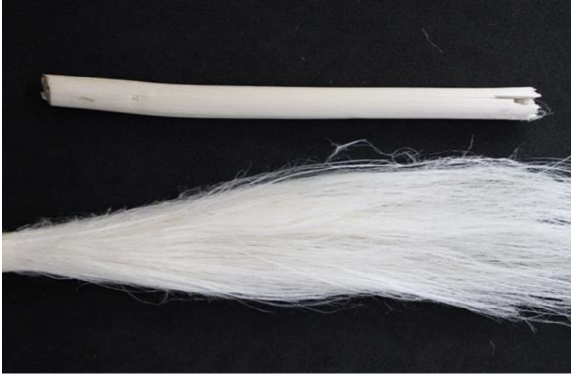
Fig. 6: Examples of hemp products after anaerobic digestion. As a result of water retting clearly separated fiber bundles without surface contamination and clean stalks (hurds) are obtained for further processing.
