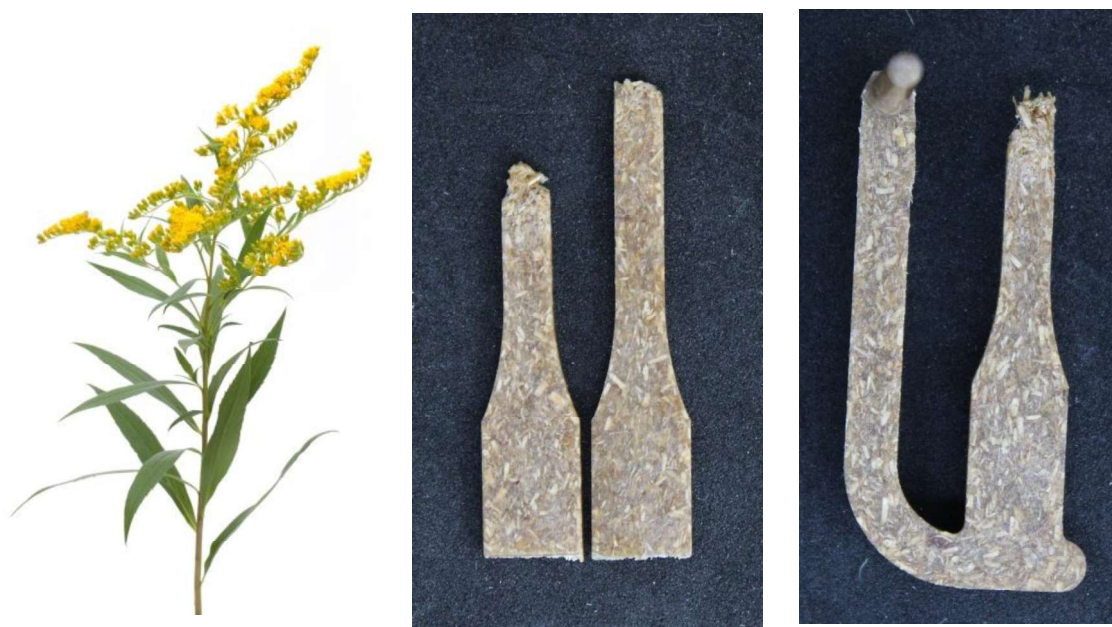
Fig. 10: Picture of goldenrod (left), tensile test bars with goldenrod (right)
