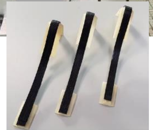
3D-printed orthosis reinforced with UD tapes
