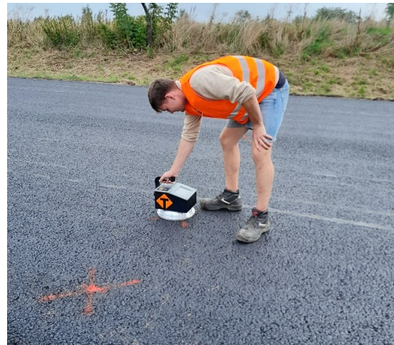
Source: Own Fig. 5: PQT probe measurements
